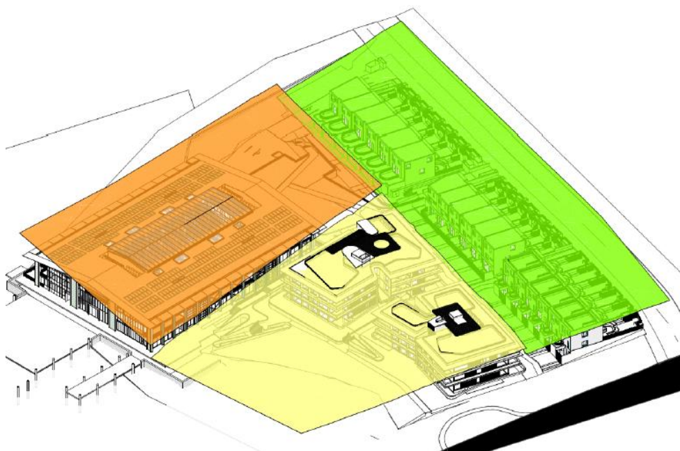
Figure 3 – Building height plane depicting elements of originally approved development encroaching above the maximum height limits
